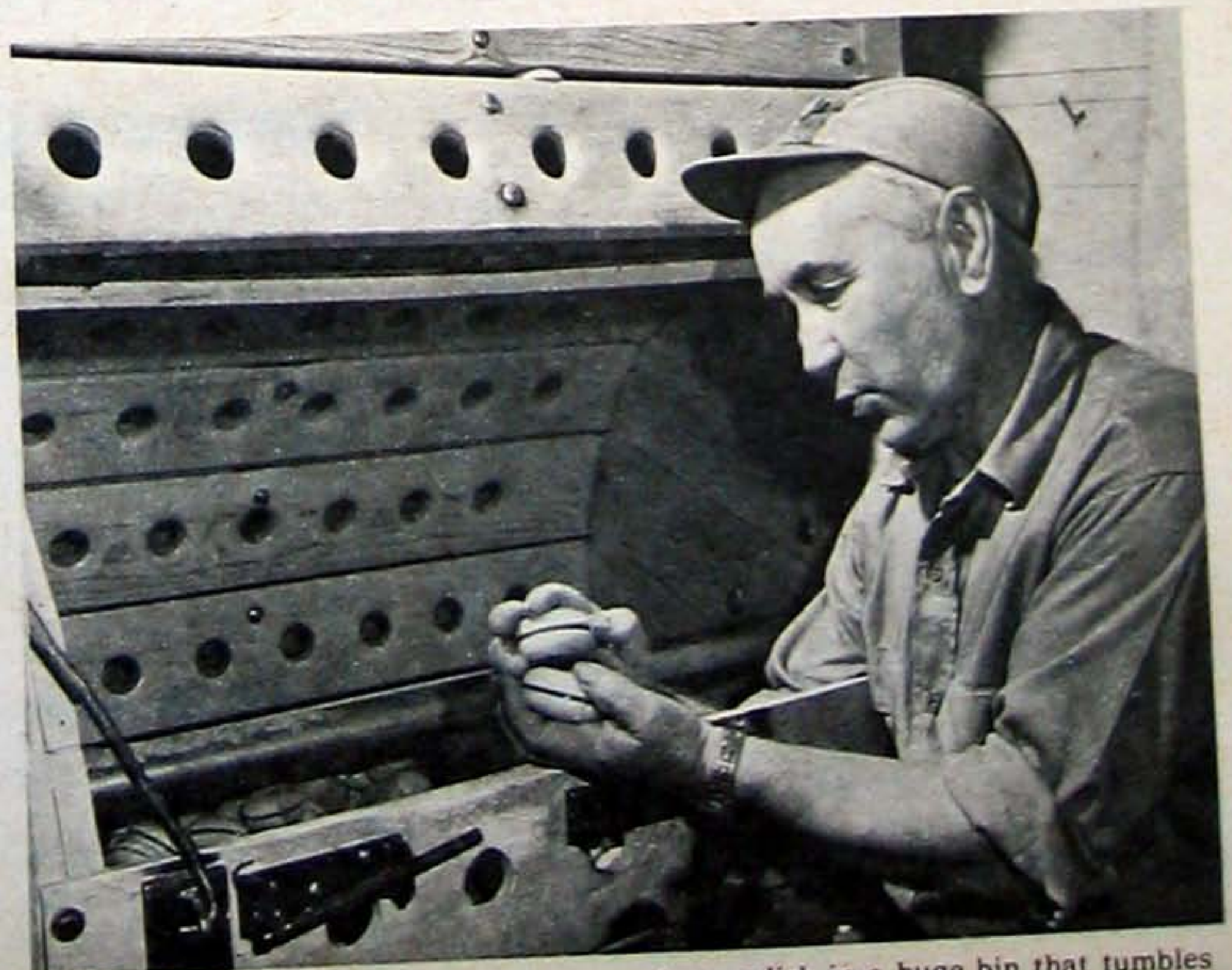
Yo-yos on a conveyor belt are automatically sprayed with paint, then dried, then given a stripe of contrasting paint in a machine watched by Benjamin Schebo.
