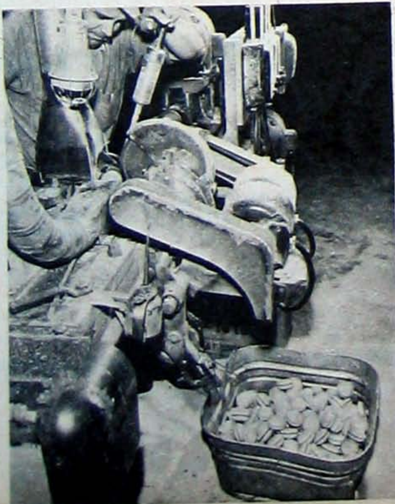
This automatic lathe, being checked by Paul Westring, is one of several that turn out the wooden tops in one piece.
