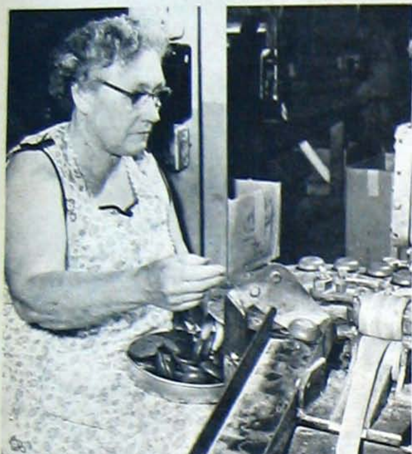
The name goes on the tops in gold leaf. Lily Mohnsen operates the stamping machine.
